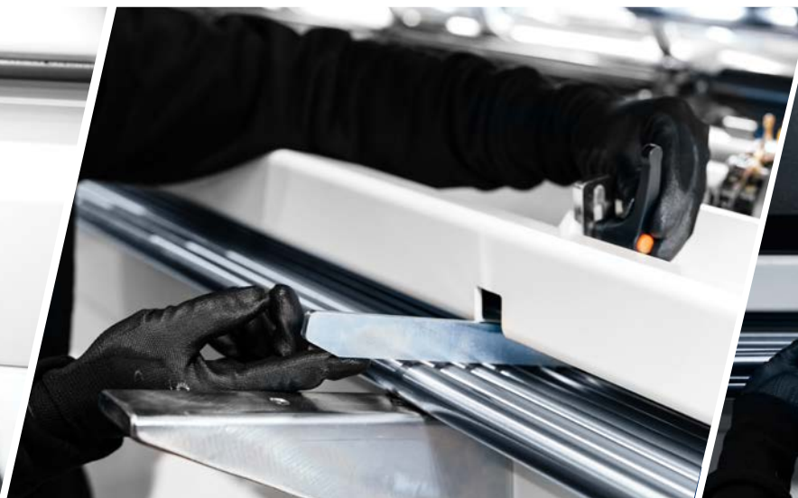
SINGLE-RACK MAGAZINE Upper guides adjustment
